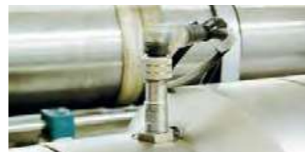
Hydraulic cylinder control with sensors
