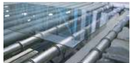
Detection of glass sheet on conveyor
