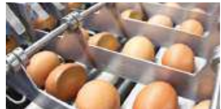
Sorting conveyor for egg packaging
